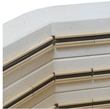
a. Detail of kiln wall with coils
